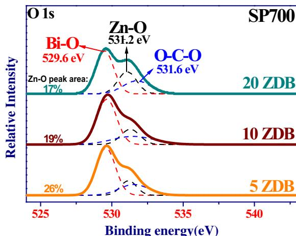
**Fig. 4.** O 1s XPS spectra and their Gaussian-resolved components for SP700 Bi<sub>2</sub>O<sub>3</sub> powders with various ZnO additions (solid line: experimental data, dashed line: Gauss fitting).
