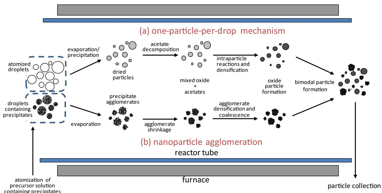
**Fig. 7.** Schematic diagram of mechanisms of  $\text{Bi}_2\text{O}_3$  powder formation in spray pyrolysis.
