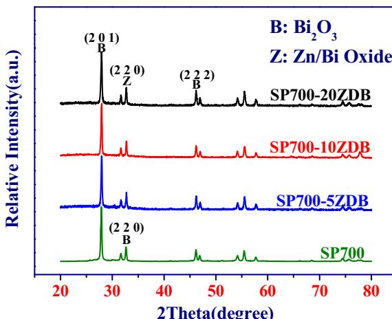
Fig. 2. XRD patterns of SP700  $\text{Bi}_2\text{O}_3$  powders as a function of  $\text{ZnO}$  addition.
