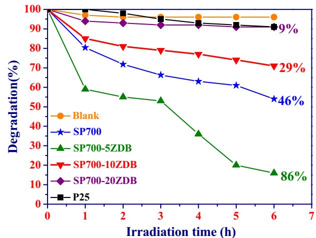
Fig. 9. Photocatalytic MO (20 ppm) degradation of SP700 Bi<sub>2</sub>O<sub>3</sub> powders under visible light irradiation as a function of ZnO addition. The concentration of catalyst suspended in MO solution is based on the same surface area.
