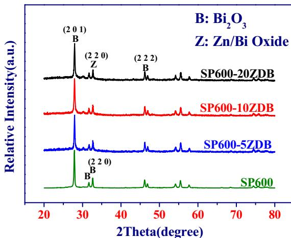
Fig. 1. XRD patterns of SP600  $\text{Bi}_2\text{O}_3$  powders as a function of  $\text{ZnO}$  addition.
