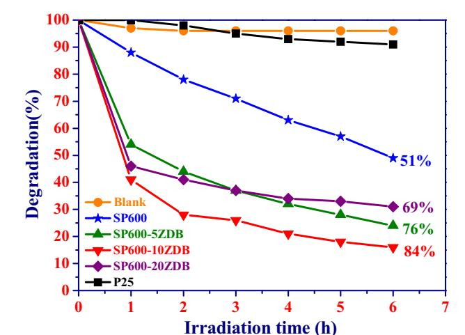
Fig. 8. Photocatalytic MO (methyl orange, 20 ppm) degradation of SP600 Bi<sub>2</sub>O<sub>3</sub> powders under visible light irradiation as a function of ZnO addition. The concentration of catalyst suspended in MO solution is based on the same surface area.
