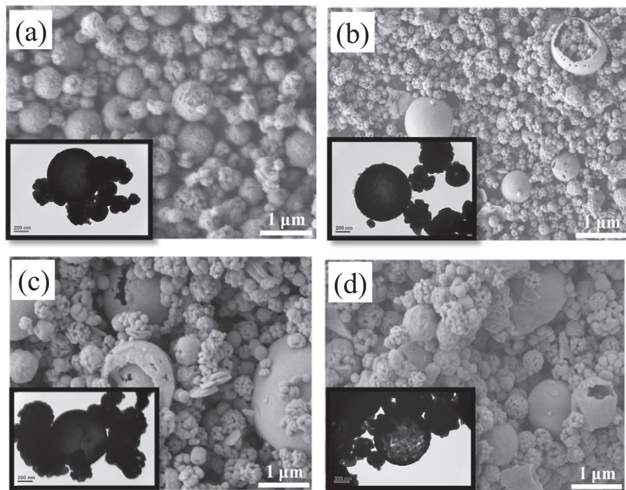
**Fig. 6.** SEM micrographs of (a) undoped SP700  $\text{Bi}_2\text{O}_3$  powder, (b) 5 mol%, (c) 10 mol%, and (d) 20 mol%  $\text{ZnO}$ -doped SP700  $\text{Bi}_2\text{O}_3$  powders.
