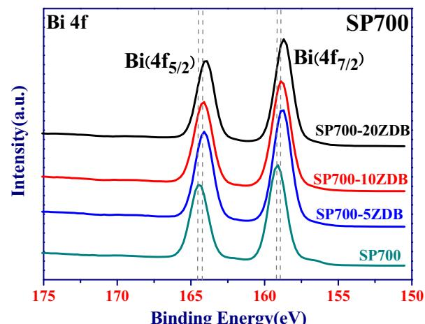
Fig. 3. Bi 4f XPS spectra for SP700  $\text{Bi}_2\text{O}_3$  powders as a function of  $\text{ZnO}$  additions.
