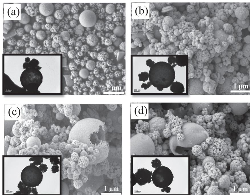
**Fig. 5.** SEM micrographs of (a) undoped SP600 Bi<sub>2</sub>O<sub>3</sub> powder, (b) 5 mol%, (c) 10 mol%, and (d) 20 mol% ZnO-doped SP600 Bi<sub>2</sub>O<sub>3</sub> powders.
